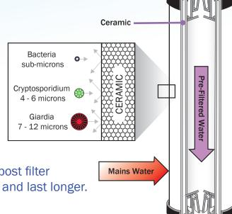
◆ The ceramic pre-filter protects the carbon block post filter cartridge, allowing it to function more effectively and last longer.
