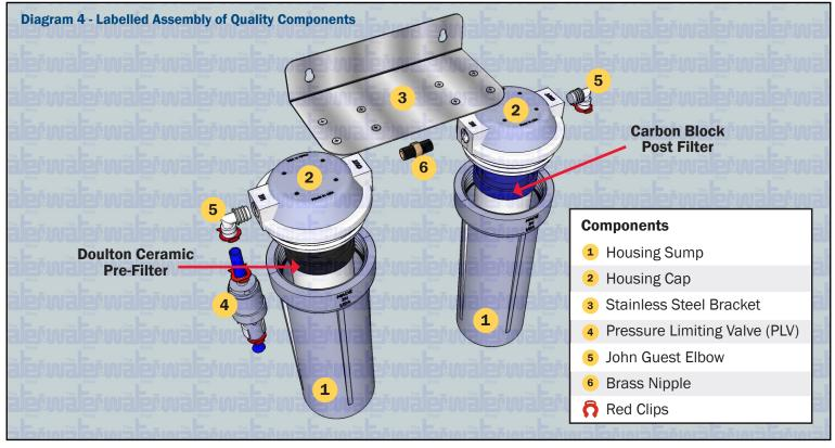
**NOTE:** Carbon cartridges may contain a small amount of carbon fines (very fine black powder). Hence a new cartridge. after installation, should be flushed with sufficient water to remove the fines before using the water.
